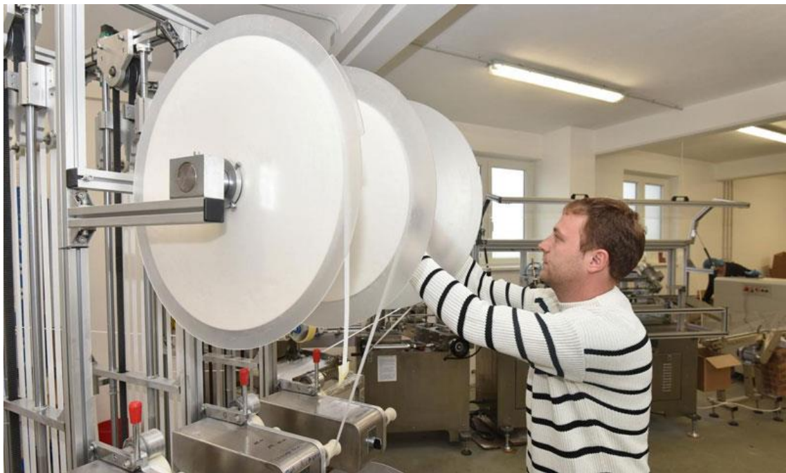
Picture 2. Part of a straw making machine
